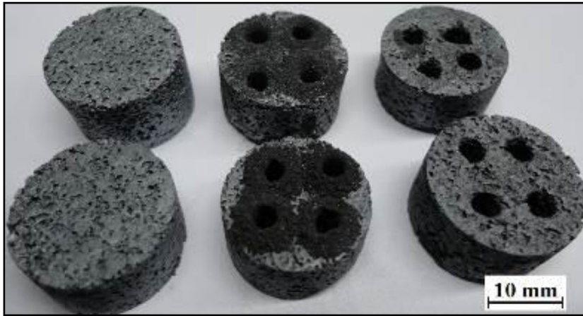
Figure 4. Photograph of the steel foams before and after drilling operations (non-machined (left), chips on the machined workpiece (middle), machined workpiece (right)).
