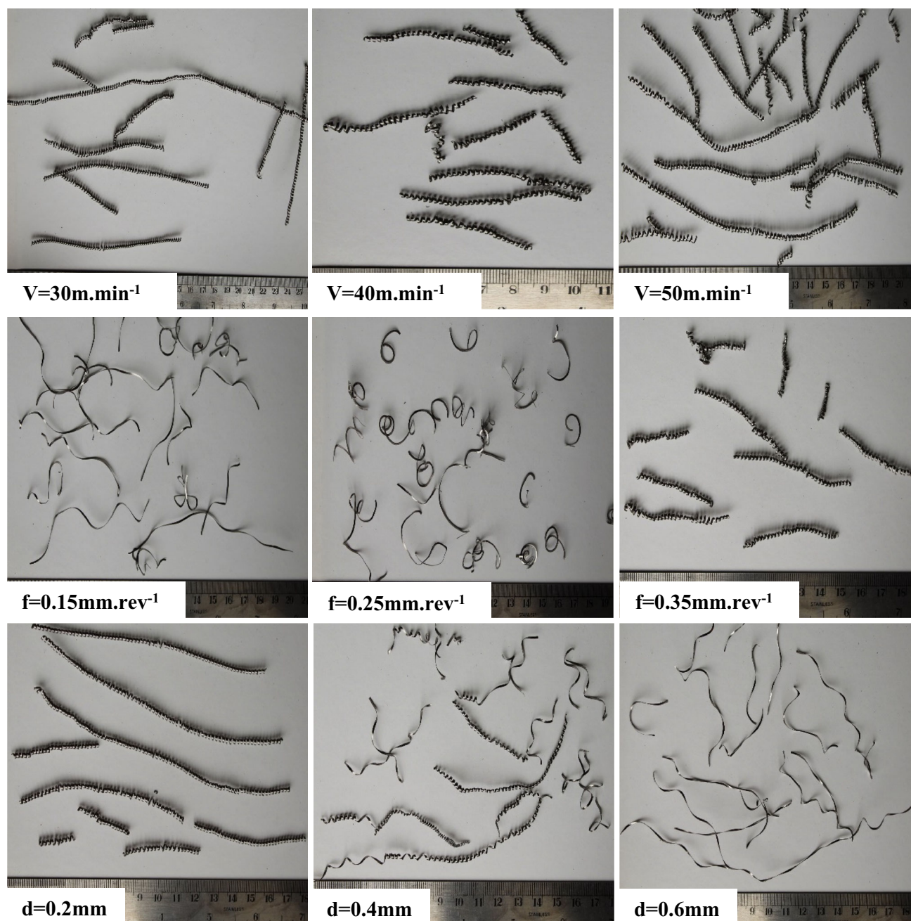
Fig. 12 Effect of the cutting speed, feed rate and depth of cut on the chip morphology turned with uncoated insert
