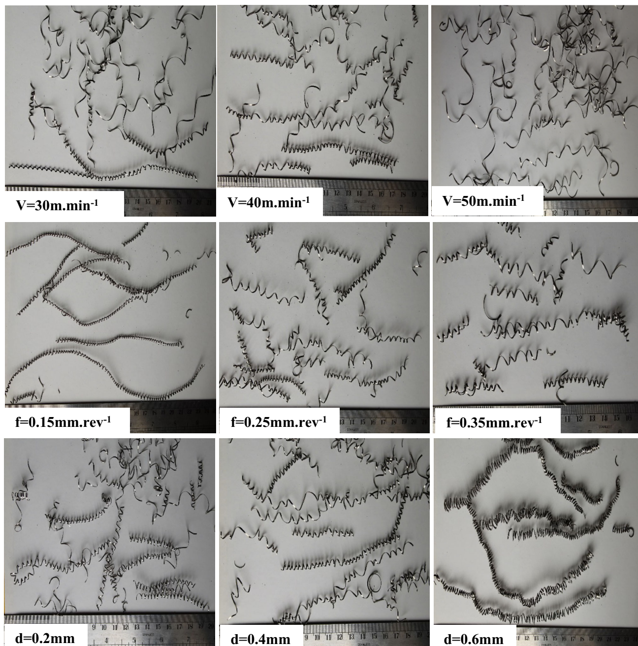
Fig. 11 Effect of the cutting speed, feed rate and depth of cut on the chip morphology turned with coated insert
