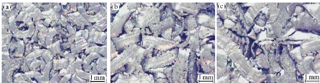
Figure 4. Typical morphologies of the porous specimens produced using the mean chip sizes (a) 4 mm, (b) 6 mm and (c) 8 mm.
